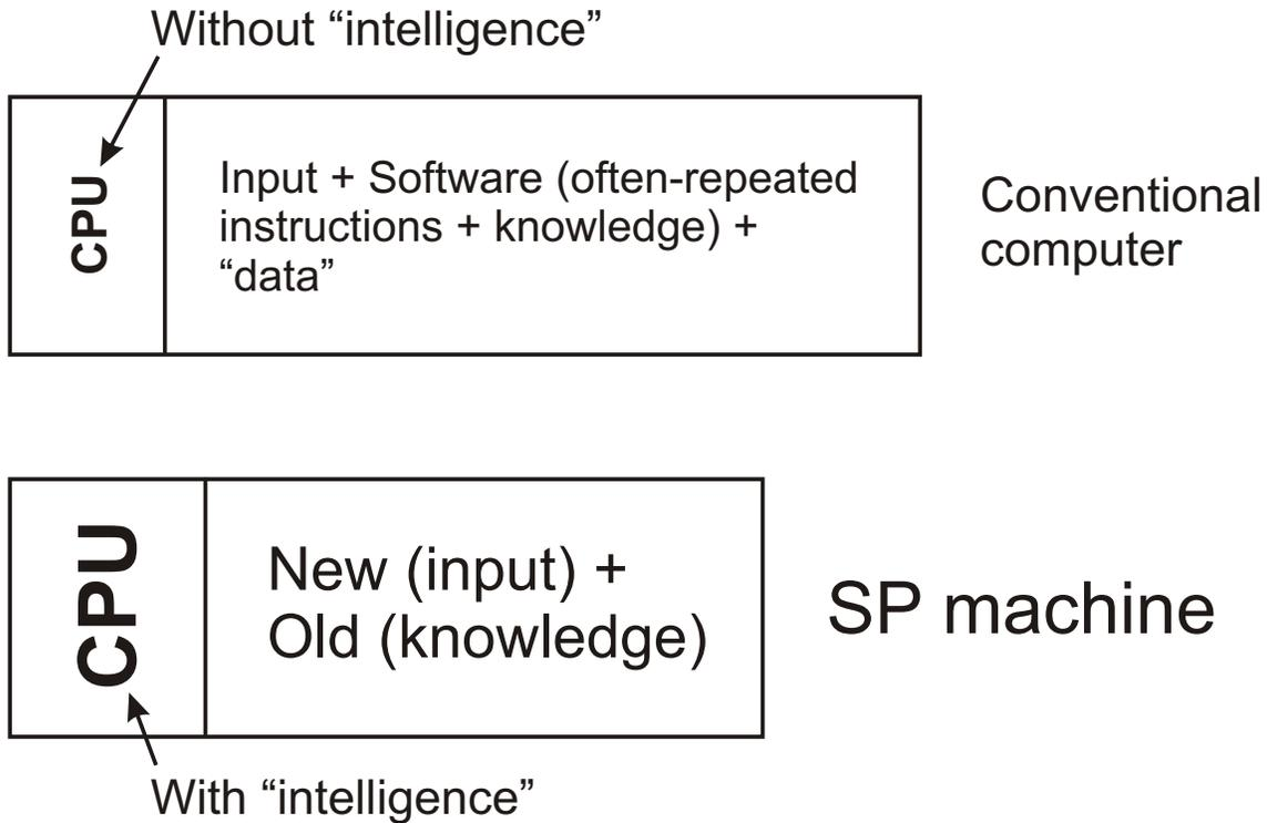
Fig. 1. Schematic representations of a conventional computer and the proposed *SP machine*, showing potential benefits in terms of simplification, as discussed in the text. Adapted from Figure 4.7 in [7], with permission.
